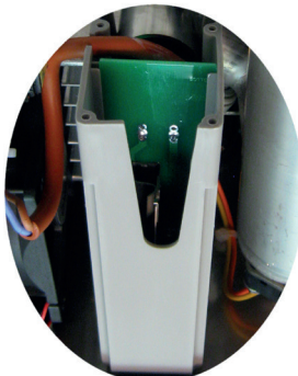
Remove Ceramic element from the housing.
