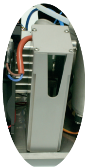
Remove 4 screws from the cover of the ceramic element housing.
