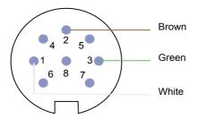
DIN-plug male Solderside Yellow and grey not connected
